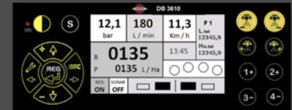
The black & white rate controller DB3610 is, apart from being a spray computer, as well a control box for up to 4 sections operating unit, and two hydraulic pistons.
