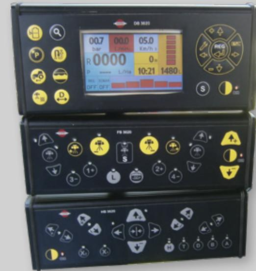
Above picture shows the DB3620 color screen with the fluid box FB3620 under it, followed by the hydraulic box HB3620.
