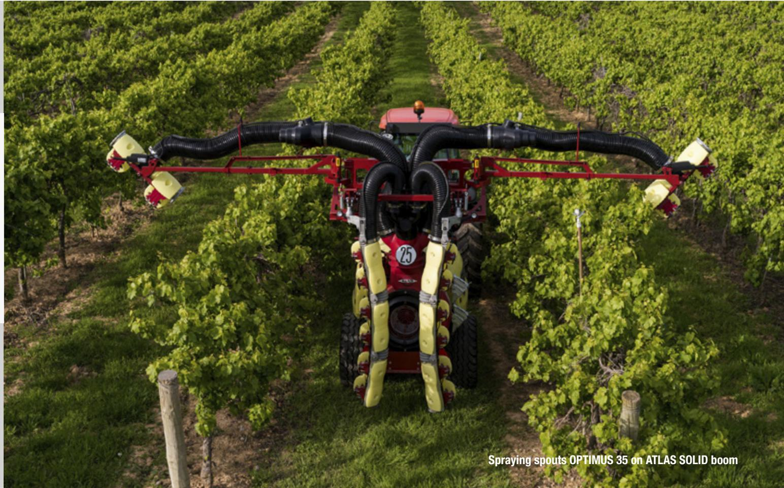
Spraying spouts OPTIMUS 35 on ATLAS SOLID boom
