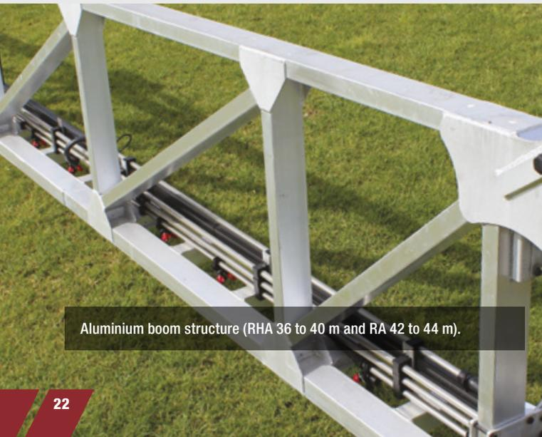
Aluminium boom structure (RHA 36 to 40 m and RA 42 to 44 m).
