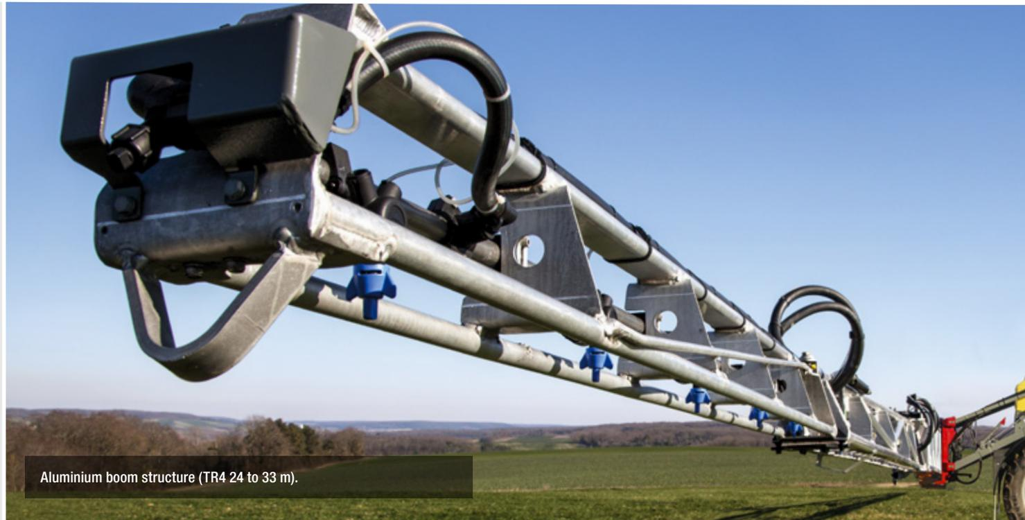
Aluminium boom structure (TR4 24 to 33 m).
