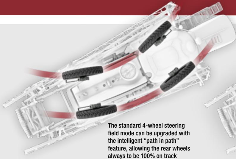
The standard 4-wheel steering field mode can be upgraded with the intelligent “path in path” feature, allowing the rear wheels always to be 100% on track
