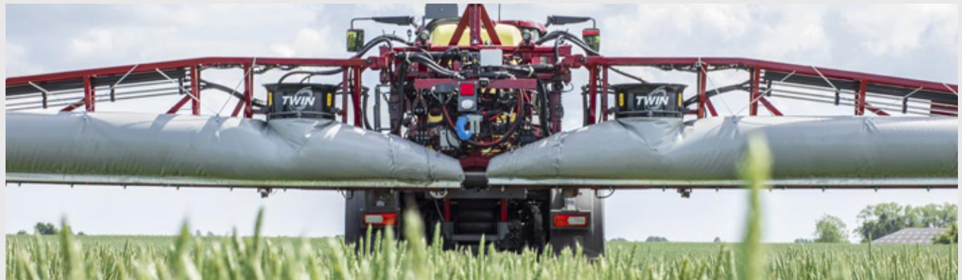
The Air-assisted TWIN FORCE boom employs the world's best system for spray control. Two powerful blower units provide air to the left and right boom sides.
